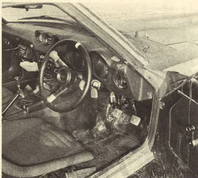
A comfortable interior with well-planned controls but some lack of stowage space for odd essential items. The special seats are non-reclining; Willans full harnesses are fitted. Note the high windscreen washer post on the scuttle
